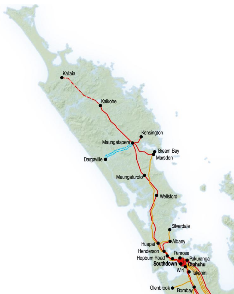
Figure 1: Upper North Island 220 kV and 110 kV network
